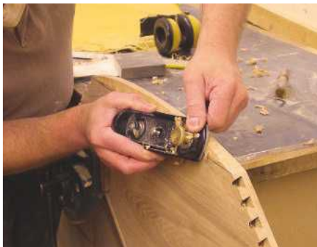
▲ Pic.12 Bandsaw the curved front edge to the top panel to shape. Then plane it smooth and create the bevel
